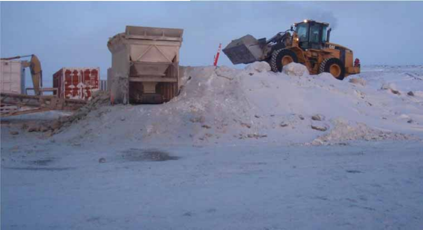
Photo 6: ~IT loader placing FCM into hopper at FCP.
