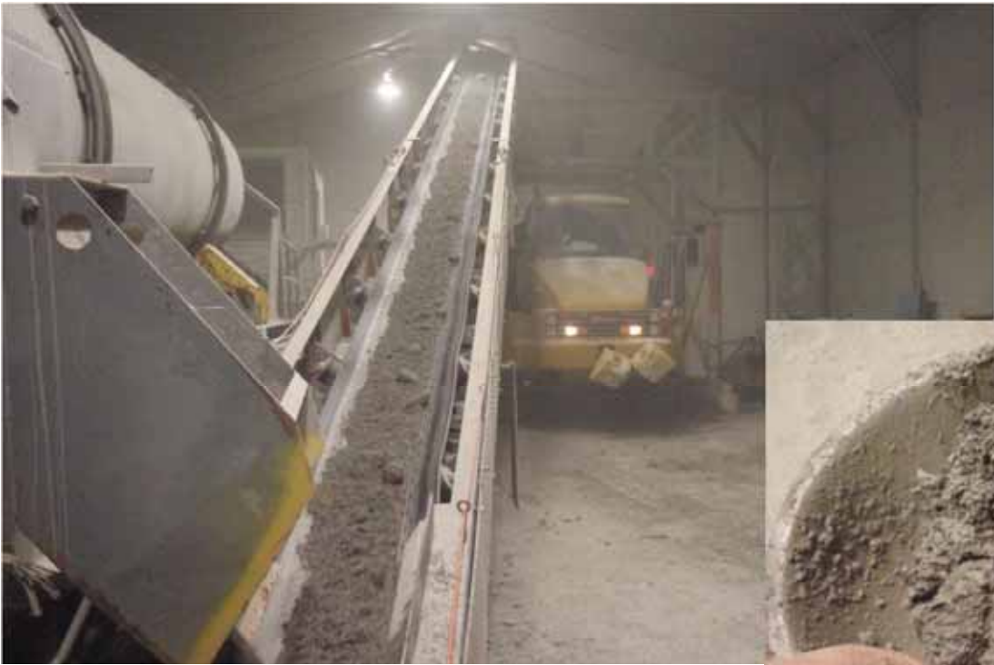
Photo 4: ~ View of FCM at FCP chute. Note this photo was taken at a time when a higher frequency of frozen lumps was being noted in the FCM. Less lumps were noted in later loads and on night shift.
