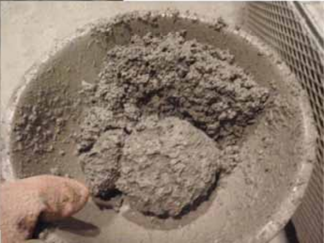
Photo 5 (bottom center): ~ Close up example of unsaturated frozen lumps observed in the FCM. A higher frequency of lumps was noted on dayshift placement however, night shift appears to have minimal lump frequency. Typically a slightly lower lump frequency was observed at the dam as FCM sits warm and heaped in the trucks before being dumped.
