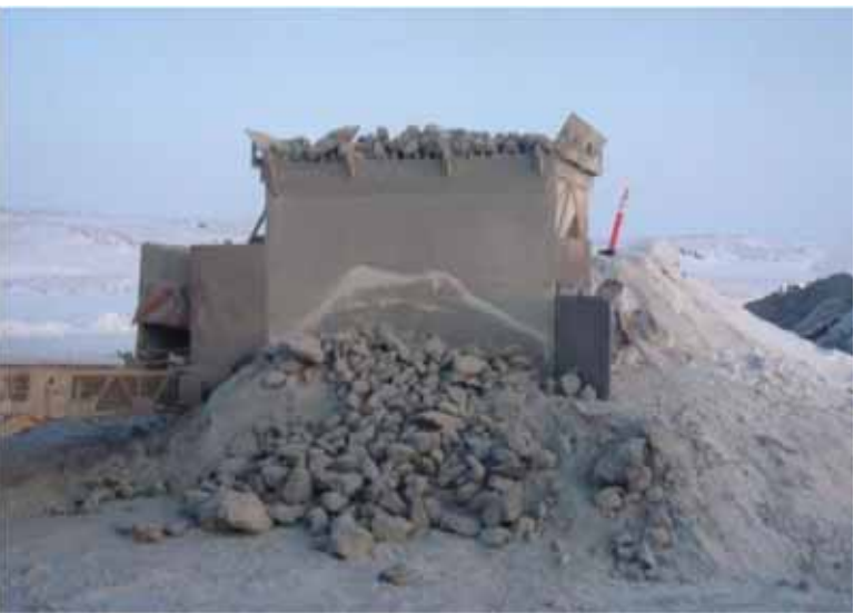
Photo 3: ~ View of frozen lumps that have been pushed of grizzly bars as FCP hopper.
